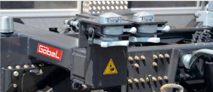
Doppelte Twistlocks in stabilem Liftadapter (Li-Version)
